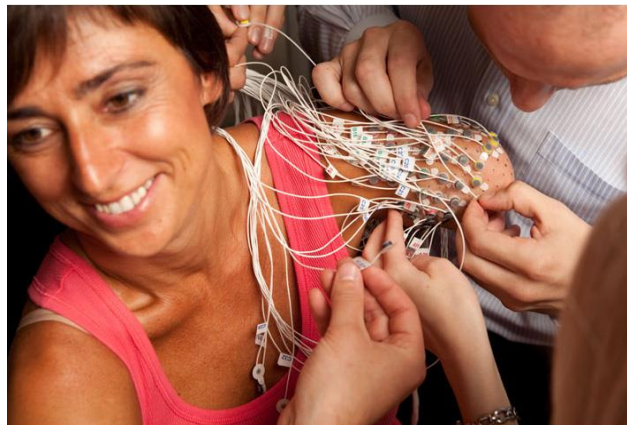
Figure 4: Example of a non-standard micro-electrode EMG configuration.
