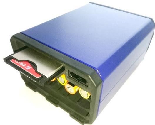
Figure 10: Porti with half-inserted Card Adapter
